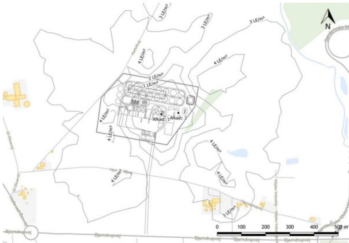
Figure: Odor propagation map. The map illustrates the biogas plant's odor contribution using isolines with a resolution of 1 LE/m 3 . The illustrated odor contribution is the 99% fractile from the biogas plant's odor sources, simulated over 10 years.
